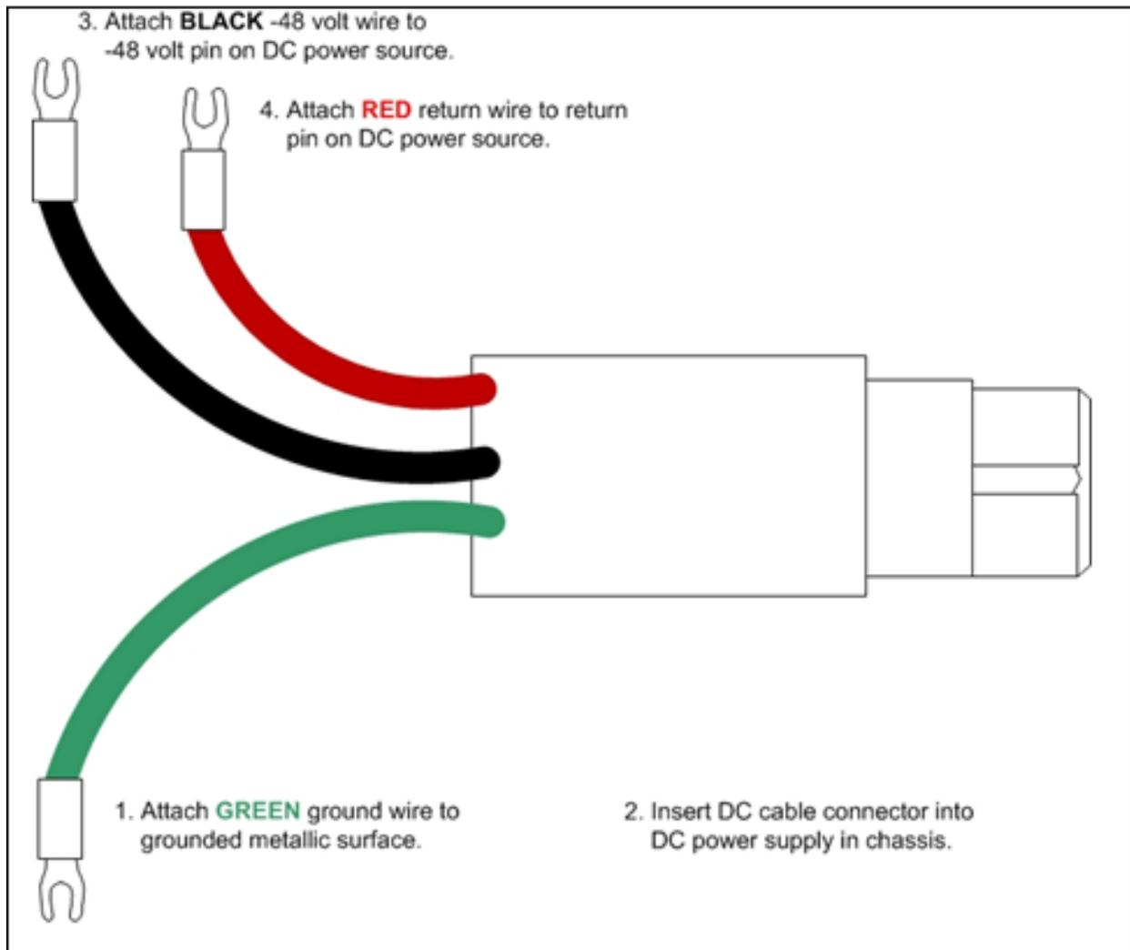
**FIGURE 8** DC Power Supply Cables
