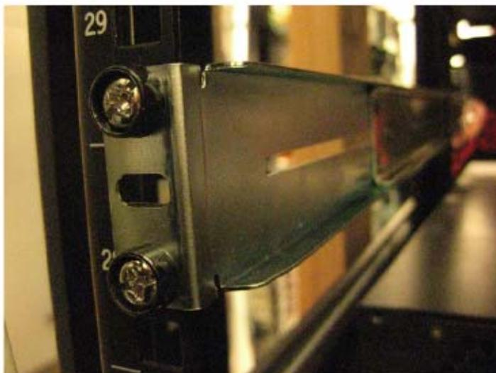
5. Tighten the two hex nuts on the outer rail to secure the rail at its extended length.
