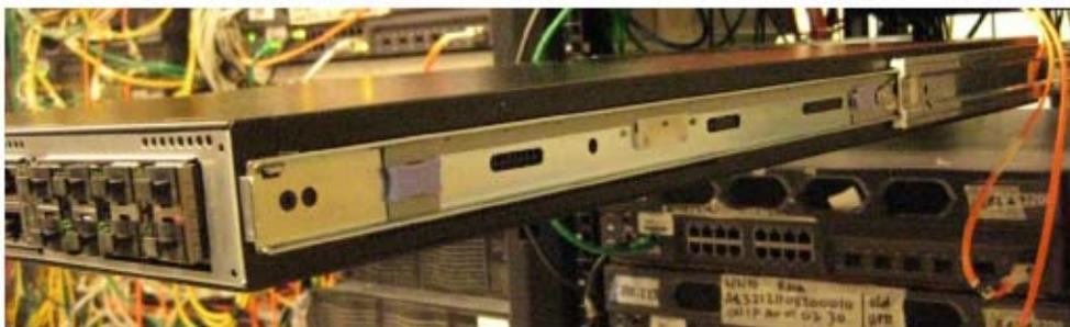
3. Slide the chassis toward the rear of the rack until the inner and middle rails lock together.
