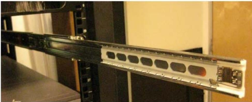
2. With the front of the chassis facing you, lift the chassis and carefully insert the inner rails attached to the chassis into the extended middle rails.
