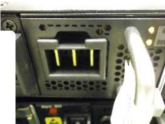
**FIGURE 6** Example of DC Power Supply (Assembled - Cable Inserted)
