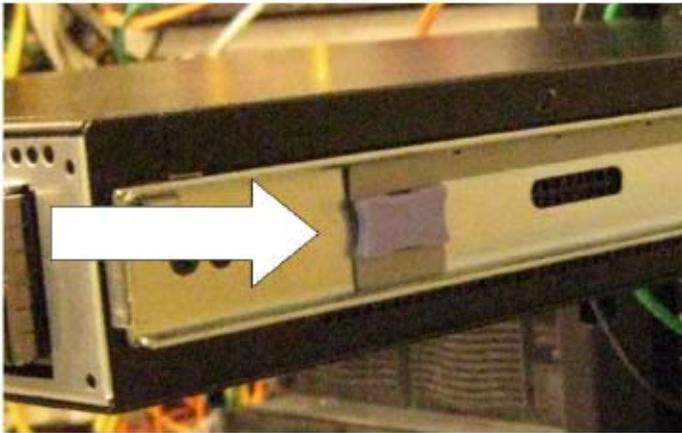
5. Carefully slide the chassis all the way into the rack. The chassis is fully inserted when the chassis handles are against the front rack posts.
