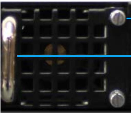
1. Loosen both screws on the right side of the module.
